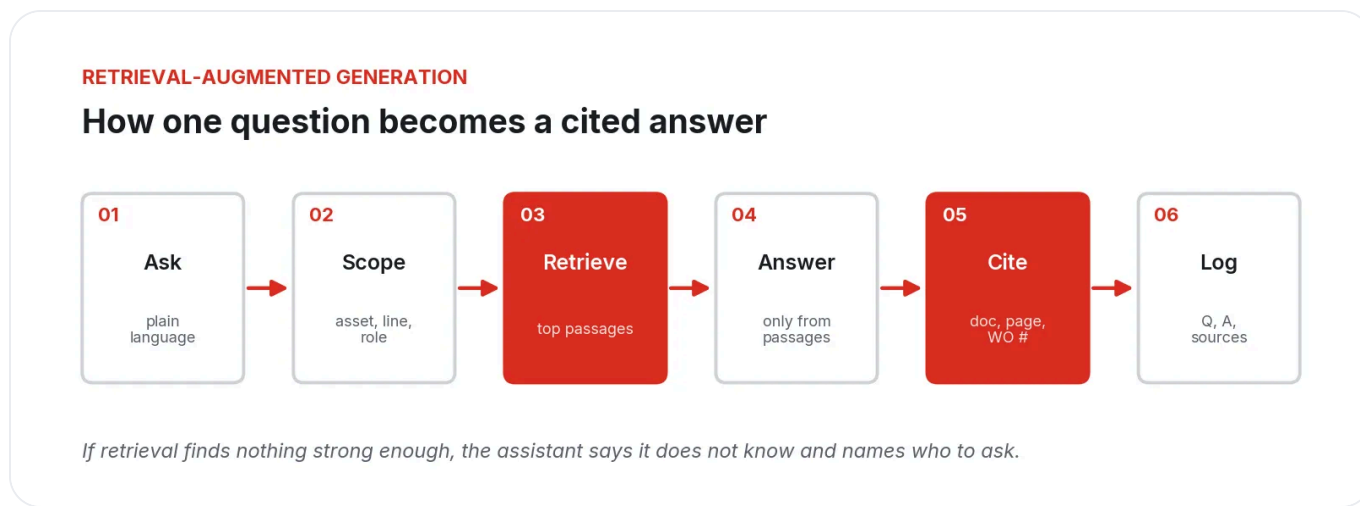
Figure 4. The retrieval-augmented answer path. Retrieval and citation are the steps that make an answer checkable at the machine.
